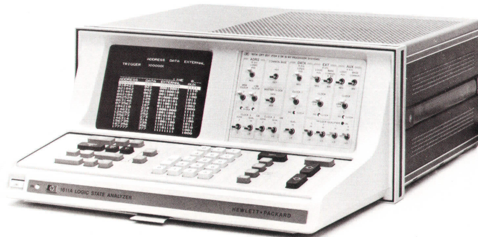
Fig. 1. Model 1611A Logic State Analyzer with the general-purpose module (option 001) installed. A keyboard and an interactive CRT display provide a "friendly" means of setting up sophisticated measurement conditions for capture and display of state flow in microprocessor-based systems. The line shown in inverse video (black on white) on the display is the trigger word that causes the lines following to be captured for storage.
