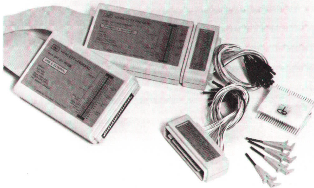
Fig. 4. The versatile probing scheme for the 1611A Opt 001 permits a variety of methods for connecting the analyzer to the unit to be tested.
