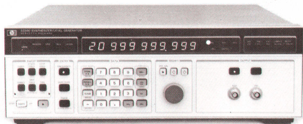
Fig. 1. Model 3336A/B/C Synthesizer/Level Generator (3336C shown) generates precise frequencies and levels over a frequency range of 10 Hz to 20.999 999 999 MHz. Output levels are accurate within \pm 0.05 dB, and integrated phase noise is less than -60 dBc.
